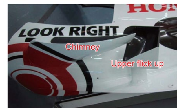
Fig. 28 Chimney and upper flick-up
